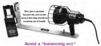
Use the Spectro-UV Model VF-100 Spec-Stik™ MIL-STD verification fixture to calibrate your lamps at exactly 15 inches (38.1cm)!
