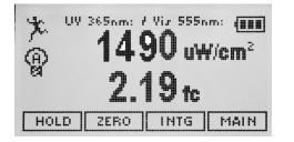
ABSOLUTE/NORMAL mode display. ZERO and INTEGRATION modes can be reached ONLY from this mode. Press MAIN to return to OPERATION/ SETTINGS display
