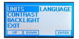
Press UP or DOWN to highlight the feature to be changed and ENTER to access the next screen, or highlight EXIT and press ENTER to return to OPERATION.
