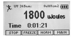
**NOTE**: While integrating, the AccuMAX will not shut off automatically after 60 minutes as it would in other modes and settings. This allows the user to continue integrating for extended periods of time.
