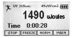
While integrating, press FREEZE to freeze and hold the displayed data. The snowflake icon will indicate that the display is static.
