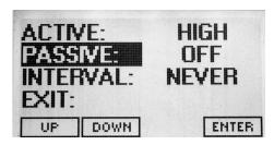
Press ENTER and then UP or DOWN to change the BACKLIGHT setting in the right column.
