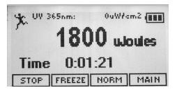
**NOTE**: While integrating, the AccuMAX will not shut off automatically after 60 minutes as it would in other modes and settings. This allows the user to continue integrating for extended periods of time.
