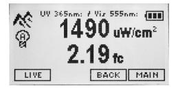
When in PEAK function, press LIVE to return to NORMAL mode, or press BACK to return to the previous HOLD screen, and press BACK again to return to NORMAL mode.
