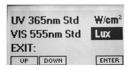
Press ENTER to return to left column, DOWN to highlight EXIT and ENTER again to access UNITS.
