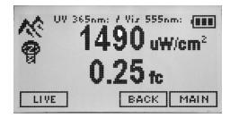
Press LIVE to return to ZERO mode, and then press NORM to return to NORMAL mode.
