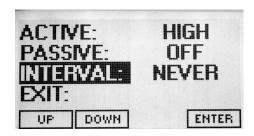
Press ENTER again to access the right column to set the length of time (60sec, 30sec, 10sec) between ACTIVE and PASSIVE operations.
