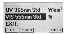
Press ENTER to highlight the right column, then UP or DOWN to change from fc to Lux.
