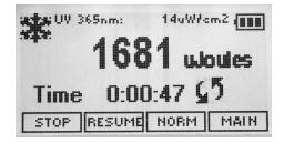
Press STOP to end INTEGRATION cycle. Press NORM to return to NORMAL mode.
